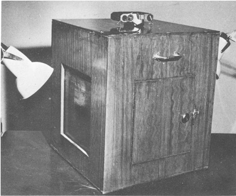
FIG. 2.— Infrared Luminescence Box showing glass cells, position of light sources, and the camera.
